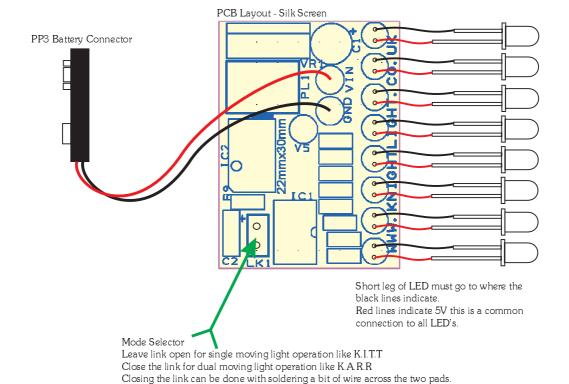
The LED's do not come fitted to the board as many customers require the LED's to be fitted away from the circuit board.
